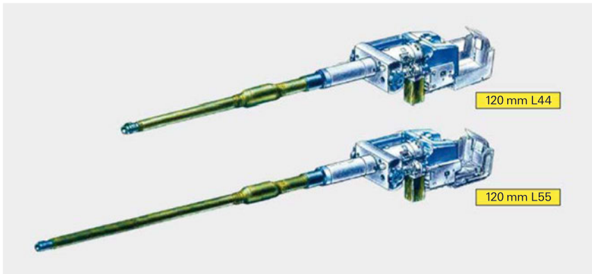
Figure 7. German Rheinmetall 120 mm smoothbore gun L44 and L55 (image credit: Thai Military and Asian Region).
