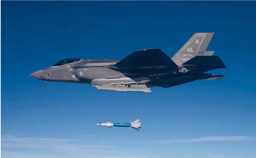
Photo 8. A Paveway II practice bomb being dropped from an F-35 aircraft (photo credit: U.S. Air Force).
